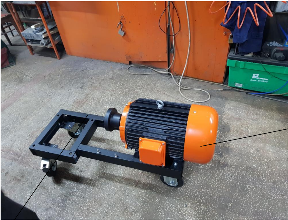
1 - Motor electric 15 kW achizitionat 2- cadru metalic realizat
