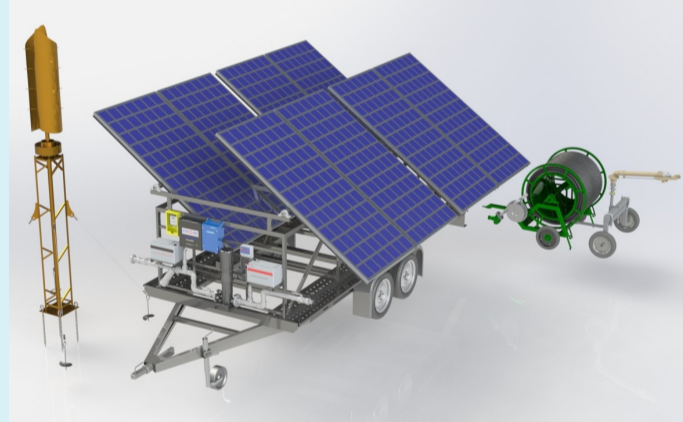
Fig. 1. Innovative energy-independent system intended for the irrigation of agricultural crops, 3D geometric model
