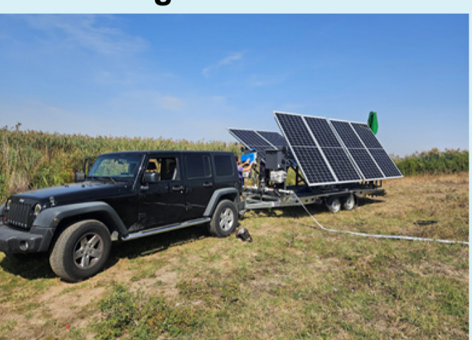
Fig. 2. Innovative energy-independent system intended for irrigation of agricultural crops, in working position
